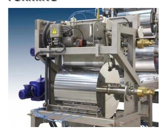
The mixture is passed through a systematic drums, where is the layer pressed into the preset dimensions. Standard can be customized thickness range from 5 to 30 mm. The machine is also suitable for processing fine, creamy and slightly aerated mixtures.
