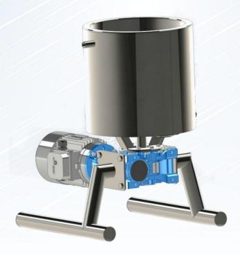
Refinining by ball mill NORMIT BALL MILL BML is achieved by mixing and friction of product with stirrer and stainless steel balls in the mixing chamber. The chamber and stirrer are made of special stainless steel with high resistance to abrasion. All parts of the machine are easily removable for easy cleaning and maintenance. The elimination of the heat generated by friction in the processing of the product allows a ball mill to work with variable speed, depending on the type of product.
