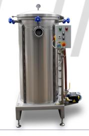
DifuVac ST vacuum diffuser is intended for performing diffusion treatment of a wide range of products, both low and high density. This vacuum liquid coater contains of sealed stationary working vessel, perforated basket, vacuum generation and maintaining system, process control system.
