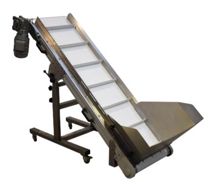
The belt conveyor support forms a very strong and quality steel structure. 50L hopper volume is at a given angle (38°), the conveyor has an adjustable height of 540-840 mm, the conveyor itself can be moved and the angle of the conveyor inclined – from 20° to 0°. Material: frame nd hopper stainless steel AISI304, belt PVC.
