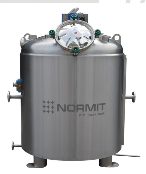
The vacuum evaporator for making sugar syrup is a cylindrical container made of high-quality stainless steel with a heating jacket and thermal insulation. The syrup is mixed using an anchor stirrer with mechanical seal. The equipment is an integral part of the semi-automatic line of the toffee mass production.
