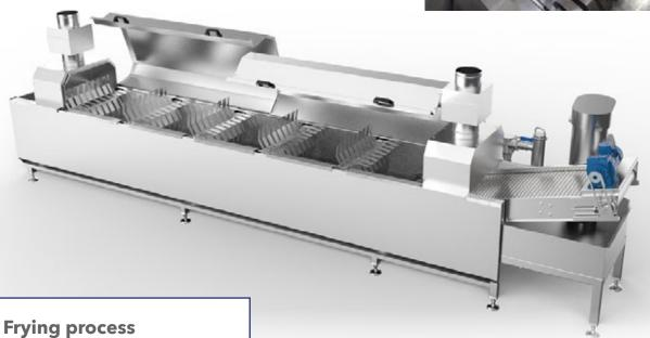
The product is fritted in a way of full immersion in hot oil. The SnackPro series of fryers do not have a conveyor belt for sliding the product. The product is shifted due to the movement of the oil pumped by the pump as well as by means of blades which not only move the product to the loading zone but also gently mix for even heat treatment.
