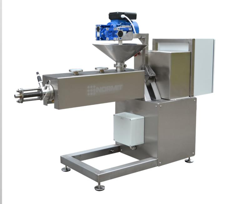
High-pressure extruder Normit HPE is designed to mix and shape various rigid, viscous and plastic products. It produces the form of the resulting product due to the slow extrusion of the product under pressure. The extruder is designed especially for processing of foodstuffs that are inapplicable for direct consumption.
