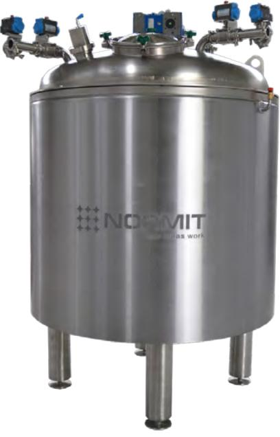
The vacuum evaporator for preparing sugarmilk-syrup is a vertical cylindrical container made of high-quality stainless steel with a heating jacket and thermal insulation. In the upper lid of the tank there is a hatch with a viewing window, a backlight, filling fittings with ball valves. In the bottom there is a temperature sensor fitting.
