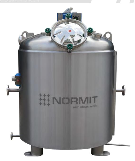
The vacuum evaporator for making sugar syrup is a cylindrical container made of high-quality stainless steel with a heating jacket and thermal insulation. The syrup is mixed using an anchor stirrer with mechanical seal. The equipment is an integral part of the semi-automatic line of the toffee mass production.
