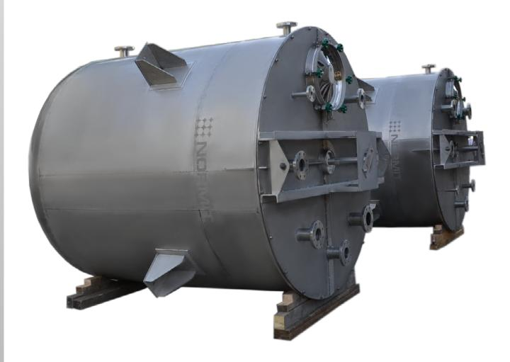
Stainless steel container with stirrer is a single-shell stainless steel vessel made of high quality stainless steel AISI 316Ti, 4 mm thick, reinforced lid with a DN 500 socket and a motorless stirrer and anchor and bearing gearbox. It is designed for use in the chemical and pharmaceutical industries, as well as for disposal of wastewater after CIP cleaning in a wide range of industries.
