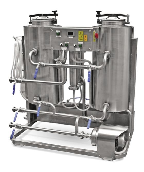
Clean-in-place (CIP) is a method of cleaning and disinfecting the internal surfaces of pipes, vessels, industrial equipment, filters, and related fittings, without disassembly.
