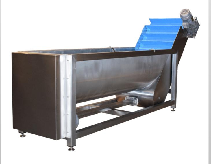
Washer with external loading conveyor UNI M is designed to effective high-performance washing of vegetables, potatoes and fruits. Purification of the product is carried out using delicate exposure to water. Is used to wash the potato, to clean seaweed from impurities or to inject substances into products.
