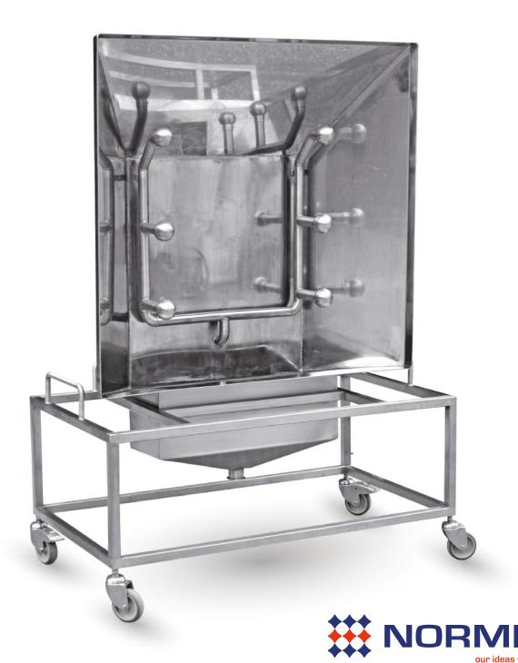
Vessel washer CEP is designed for cleaning various containers - for example z-blades mixer, which can be tilted. The washer also allows the use of steam. The device is equipped with spray nozzles for rinsing water. Mobile washing equipment for washing of various mixers with tilting bowl, boilers, kneaders and other similar equipment
